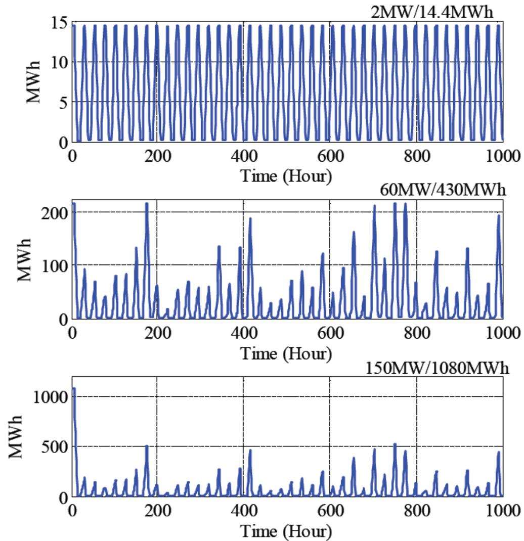
Fig. 6. State of charge profile at daily operation
