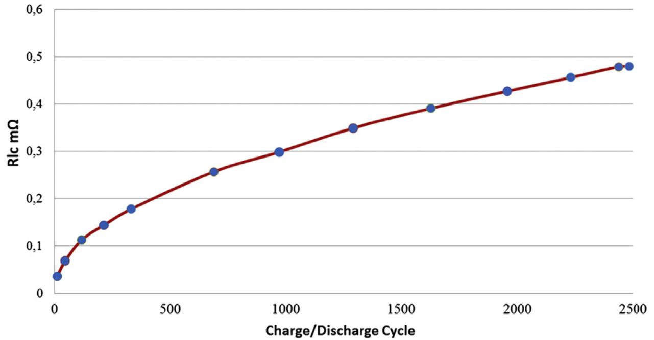
Fig. 4. Variation in internal resistance of NaS battery as a function of charge-discharge cycles.
