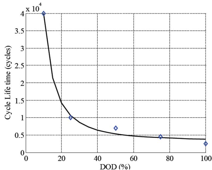
Fig. 5. Depth of discharge vs lifetime in cycles for NaS battery.
