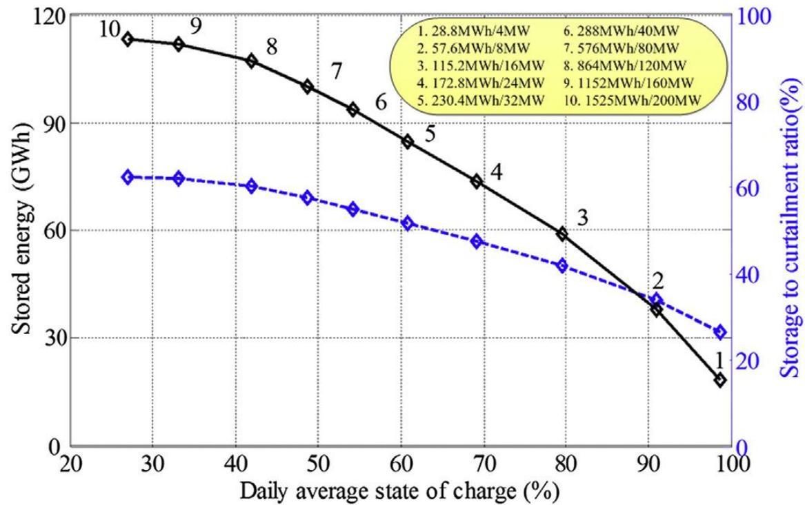
Fig. 8. NaS battery storage system performance (Scenario I).
