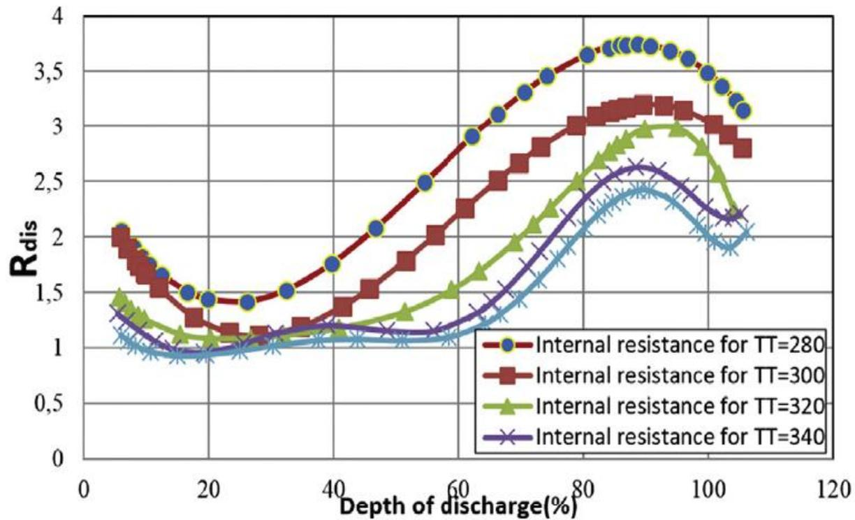
Fig. 3. NaS cell resistance in discharging mode vs DOD at different temperatures.
