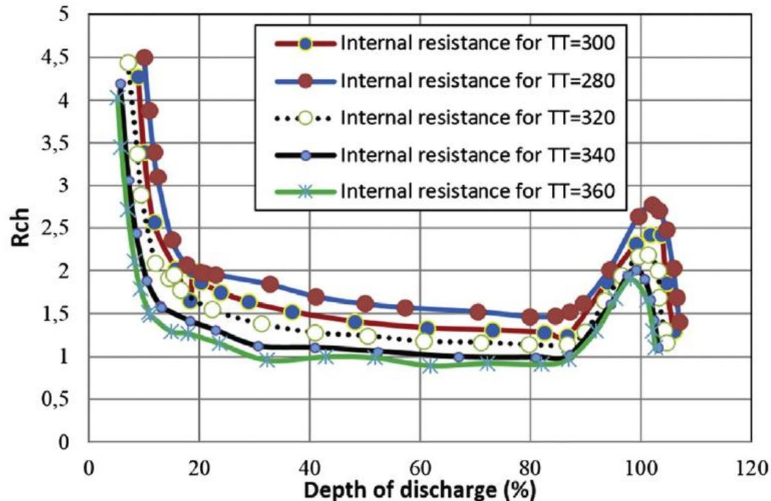
Fig. 2. NaS cell resistance in charging mode vs DOD at different temperatures.
