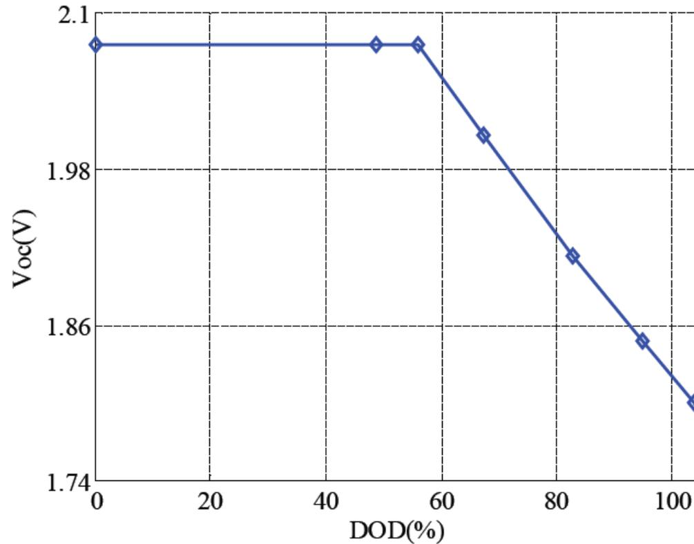
Fig. 1. Open circuit voltage as function of battery DOD.
