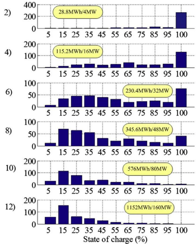
Fig. 7. DOD distribution for one year of operation as function of battery bank size.
